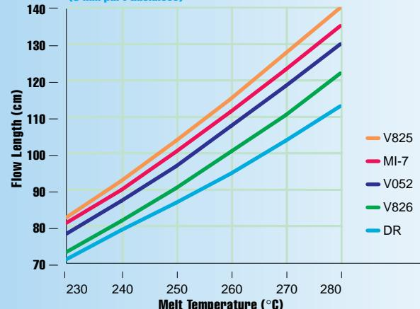
\*Flow data generated using mold filling analysis simulation. Constants of 70° C mold temperature, 15,000 psi cavity pressure and 1.0 inch<sup>2</sup>/second fill rate were used for all runs.
