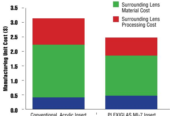
20% cost savings realized due to the elimination of part cracking during insert molding. Process yields increased from 66% to 97+%
